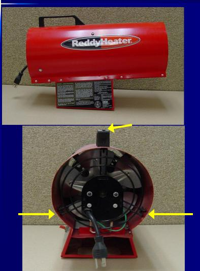
• Make sure the heater is disconnected from its gas supply and unplugged.
