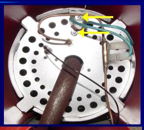
Use your 3/8" and 1/4" nut drivers to remove the bolts and nuts that hold the thermal switch in place
