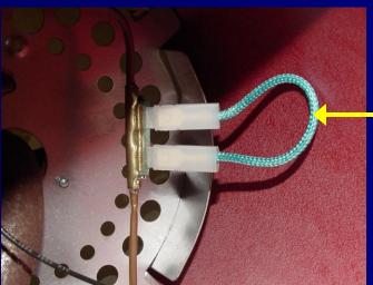
Set the thermal switch and screws aside
